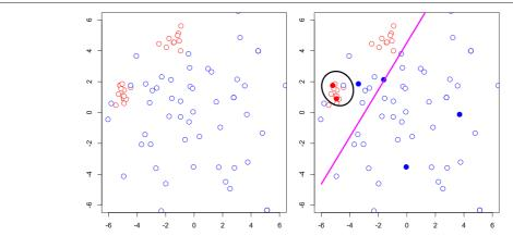
Fig. 1 Example of two-dimensional case. In the left, the blue and red open circles represent the candidates of inputs with y = 1 and y = -1, respectively. In the right, the filled circles and the curve represent the sampled inputs, the black solid line is the estimated decision boundary via SVM, and the purple solid line is the linear discriminant boundary
